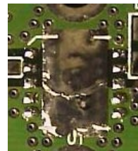
Figure 3. PCB shown with solder added to ground pad and leads.
