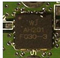
Figure 12. PCB shown with properly soldered AH201 device.
